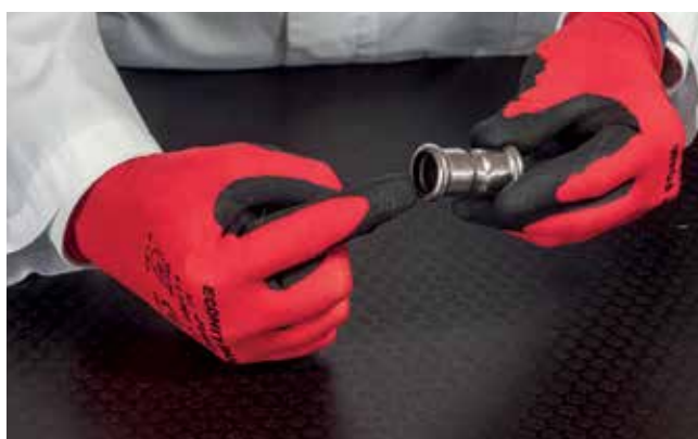
Controllo O-ring / Checking the sealing ring
